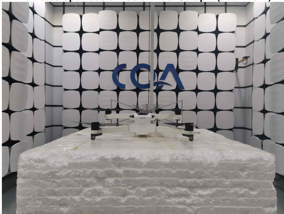
Radiated spurious emission Test Setup-1 (Below 1GHz)
