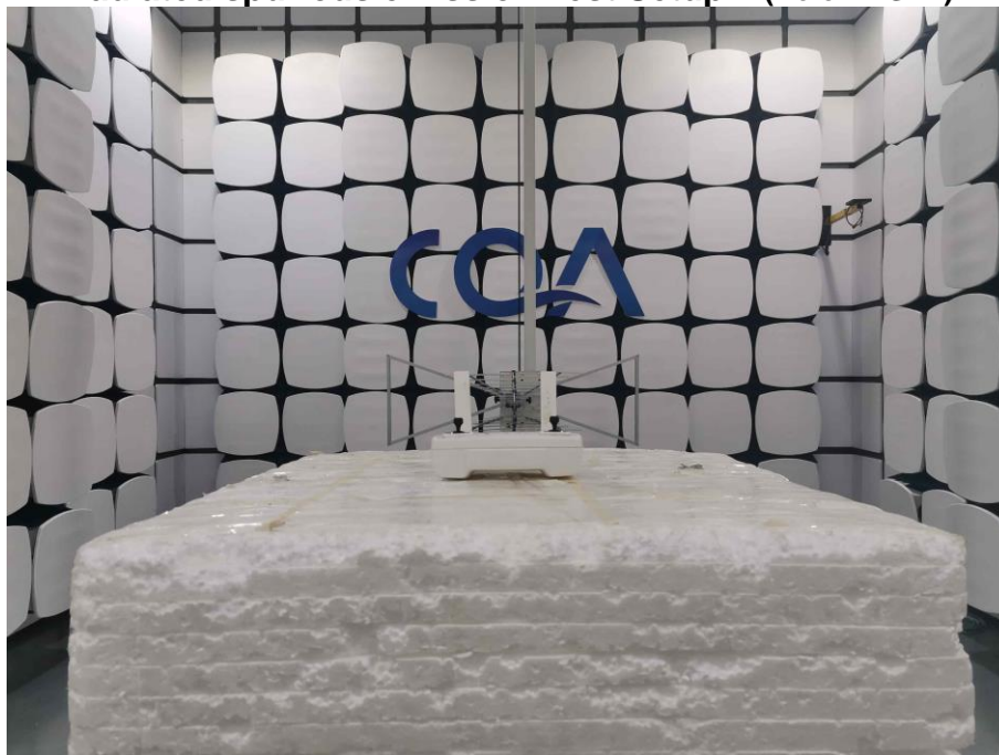
Radiated spurious emission Test Setup-1 (Below 1GHz)
